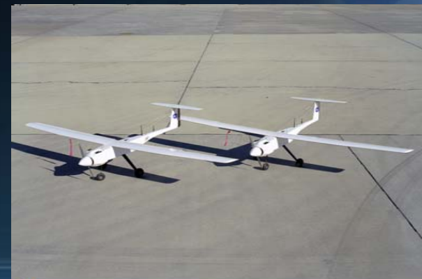
NASA Dryden Flight Research Center Photo Collection http://www.dfrc.nasa.gov/Gallery/Photo/index.html NASA Photo: EC04-0347-06 Date: November 20, 2004 Photo By: Tom Tschida Two identical RnR Products APV-3 aircraft validated cooperative flight control software in the Networked UAV Teaming Experiment at NASA Dryden in early 2005.
